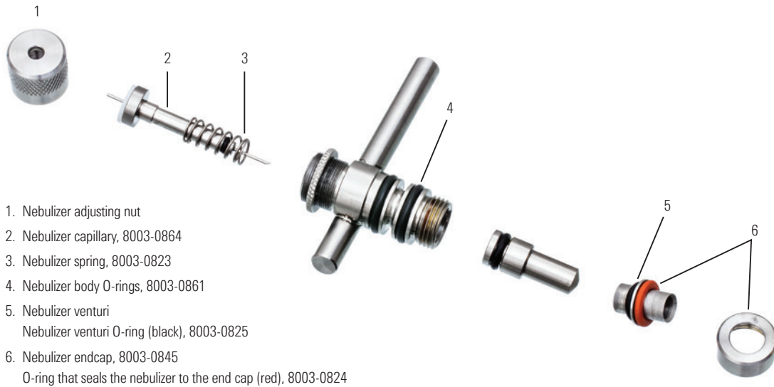
Exploded view of Nebulizer assembly, 8003-0828
