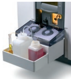
SIPS 20 Sample Introduction Pump System for flame AA
