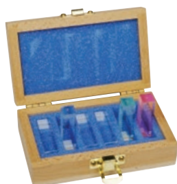
Fluorescence samples, set of six hydrocarbons in polymer blocks, 6610010300
