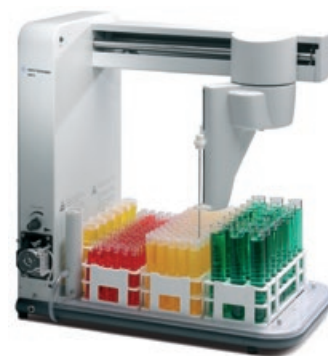
SPS 3 autosampler for AA, MP-AES, ICP-OES, and UV-Vis instruments (now replaced by the SPS 4)
